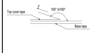
The force for tearing off cover tape is 15 to 80 grams in the arrow direction under the following conditions (referenced ANSI/EIA-481-D-2008 of 4.11 stadnard)
